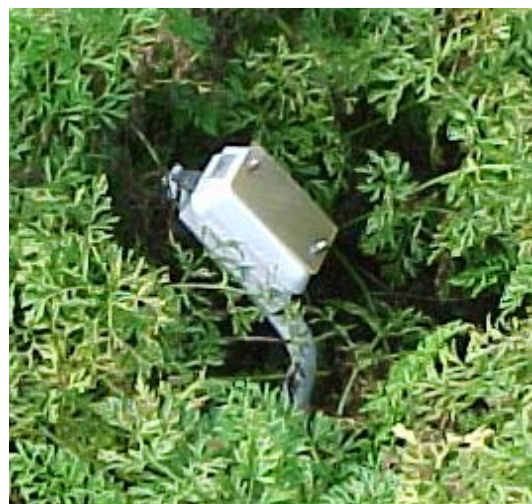
Figure 1. A leaf wetness and temperature sensor is oriented at a 45° angle facing north and located in the upper 75% of the carrot canopy.
